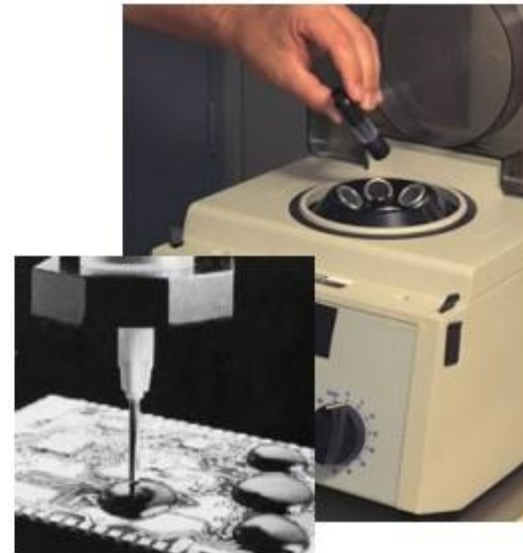
A centrifugal machine for removing air bubbles from the protective compound
