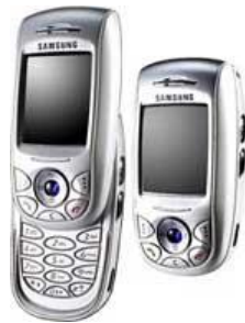
Mobile phone with a sliding part which contains a microphone and protects keyboard.
